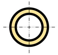
In a concentric-tube column, the mass transfer between the vertically rising steam and the liquid film, which falls downwards in a spiral, is realized. The column is therefore designed as a concentric tube.
